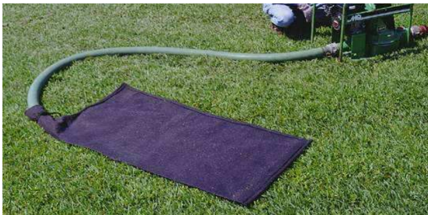
Photograph CS-2 – Example of Dewatering Bag
